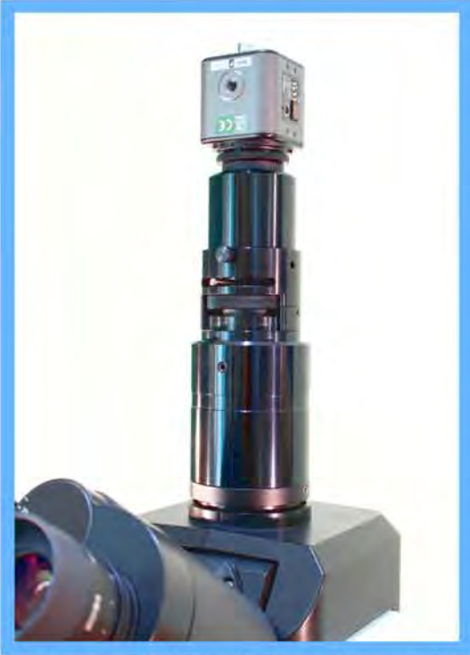
"U" bottom assembly holding M2 APO - with C-mount adapter to camera
